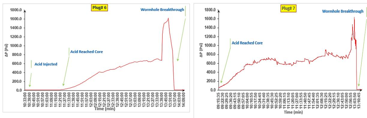
**Fig.9.** Differential pressure against time acid flooding, (a) Plug#6 flow rate 400 cc/hr , (b) Plug#7 flow rate 40 cc/hr.
