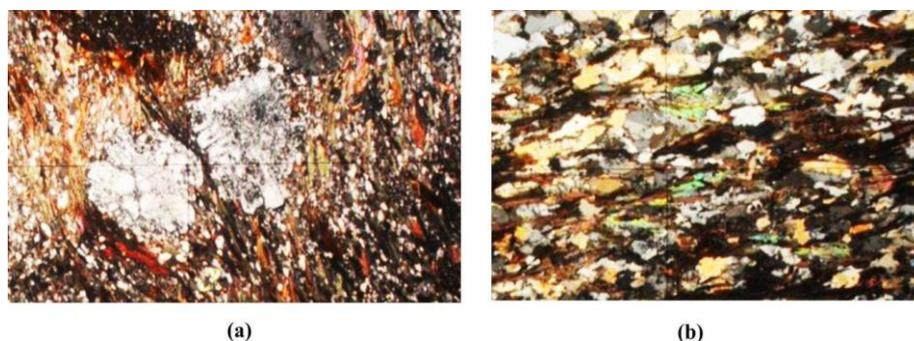
Fig. 2. A) Porphyroblastic texture of metapelites rocks (sample 1); B) Granoblastic texture of metapelites rocks (sample 3)
