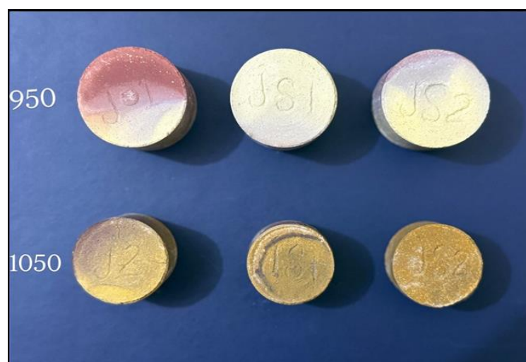
Fig. 8. Variation in the degree of efflorescence in brick samples at different firing temperatures
