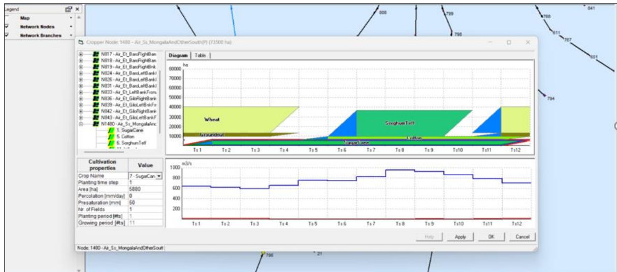
Fig. 3. Seasonal irrigation area and related water demand downstream of Mongala as the RIBASIM Model input sample
