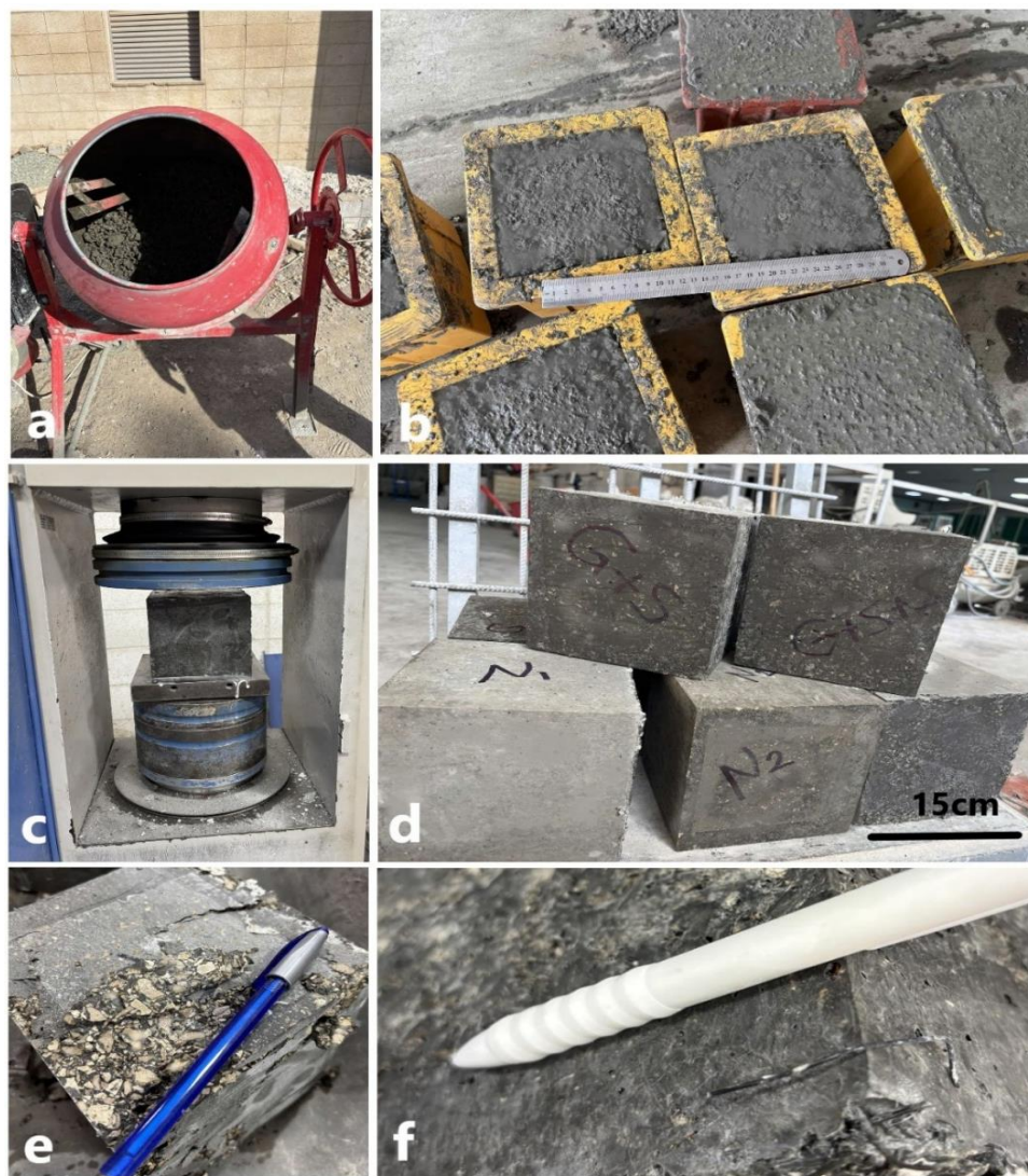
Fig.4. a) The aggregate-cement paste while mixing; b) the mixture inside the molds on the vibrator; c) the concrete cube under unconfined compressive strength; d) the concrete cubes (15cm); e) the concrete cubes after compressive strength test remained compacted with little fractures; f) After 28 days of curing, the steel fibers remained free from observable rust formation, indicating stable performance within the concrete matrix
