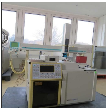
Fig. 3. Gas Chromatography (GC) instrument in the laboratory to analyze natural gas
