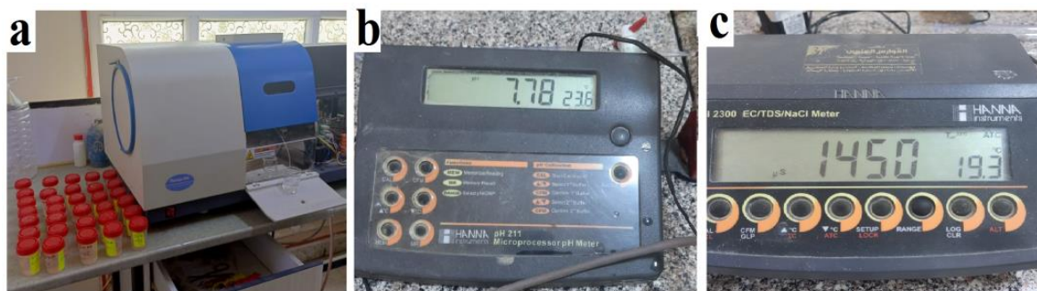
Fig.6. Atomic absorption spectrophotometer (a); pH meter (b); EC, TDS meter (c)
