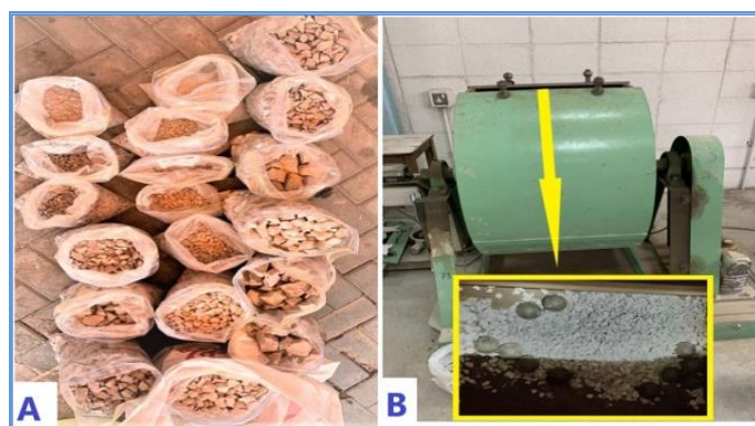
Fig. 2. LAS abrasion test A) eight aggregate samples were prepared according to Class B gradation; B) Steel drum with 11 iron balls.
