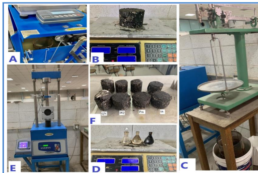
Fig.6. (a) weight of aggregate in water; (b) weight of the molded mixture in air; (c) weight of the molded mixture submerged in water; (d) specific gravity of bitumen by weight (pycnometer); (e) marshal stability test; (f) flow of the HMA moulds
