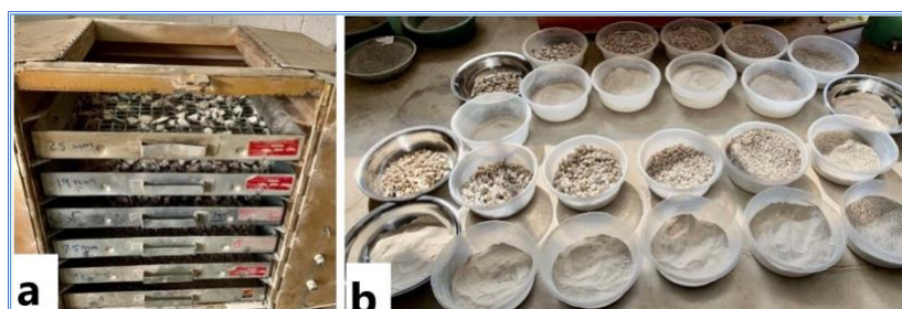
Fig.3. (a) sieve shaker machine (b) aggregate size preparation
