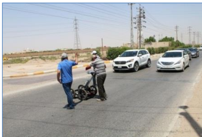
Fig. 3. GPR survey to explore the Second Phase of the Old Euphrates River in Al-Najaf Al-Ashraf Governorate for track 1
