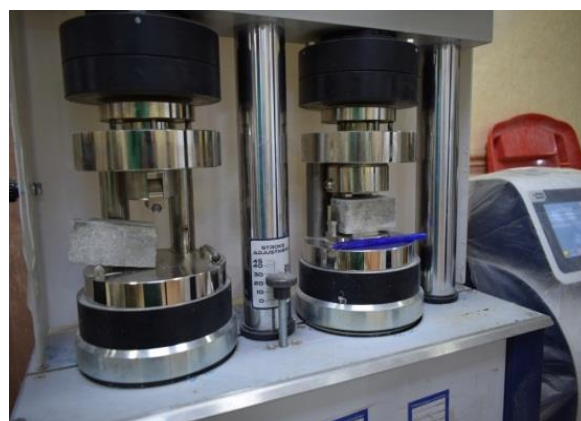
Fig. 3. Testing the compressive strength of the samples.
